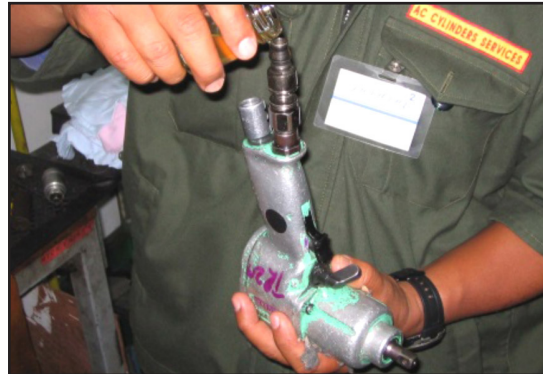
Using Chesterton 652 Pneumatic Lubricant to clean the deposits inside the air tool.
