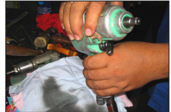
Pneumatic tool internal residues are removed with Chesterton 652.
